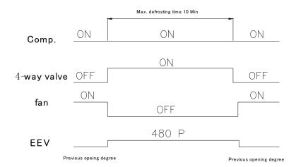
EEV stay 480P opening degree when defrosting, 4min after defrosting EEV start regulating
