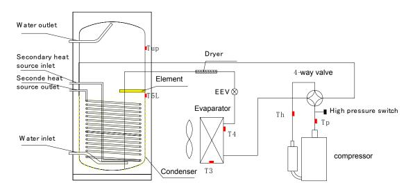
Compressor: Mitshubishi RB233GRDC, R134a; Element: located in the mid of tank, 3000W/230VAC;
