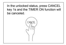
2.2.4.7 **TIMER ON and TIMER OFF:** Users can set up a running start time and a stop time. When the start time is earlier than the stop time, the unit will run between the set time. When the start time is later than the stop time, the unit will run between the start time today and the stop time next day.
