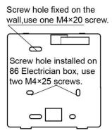
Adjust the length of two plastic screw bars in the accessory to be standard length from the electrical box screw bar to the wall. Make sure when install the screw bar to the electrical box screw bar, make it as flat as the wall.
