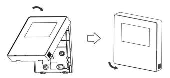
Correct install the back cover and firmly buckle the front cover and back cover, otherwise will make the front cover drop off.
