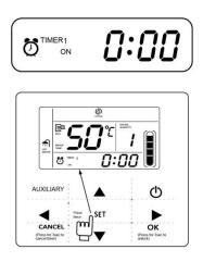
✓ At this time the hour of the clock will flash, which means the current setting is the hour of Timer 1 on, press the ▲ or ▼ to adjust, press ► key when finished, and then the minute of the clock will flash, which means the current setting is the minute of Timer 1 on, press the ▲ or ▼ to adjust, press ► key when finished, the LCD will display as the following:
