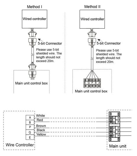
There are two methods to connection between wired controller and main unit.
