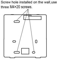
Use two M4x25 screws to install the back cover on the 86 electrician box, and use one
