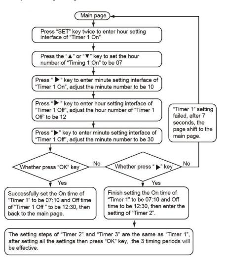
During any period of timing setting to press **OK** key, the timing periods which have been set will be effective (only if the on and off of one timing period have been set, the setting is effective). Check timing information: to check the timing which has been set, press  $\blacktriangleleft$  or  $\blacktriangleright$  key under main page, the on and off time of Timer 1, Timer 2 and Timer 3 will be displayed in turns.
