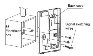
Use cross head screws to fix the wired controller bottom cover in the electric control box through the screw bar. Make sure the wired controller bottom cover is on the same level after installation, and then install the wired controller back to the bottom cover. > Over fasten the screw will lead to deformation of back cover.
